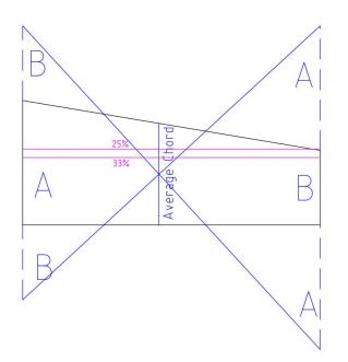
We start by making a drawing of our wing (half will do). If our wing has a rounded tip, square it off. Graph paper works fine. If you're comfy with CAD software, that works fine, too (it better 'cause that's what I use!).
